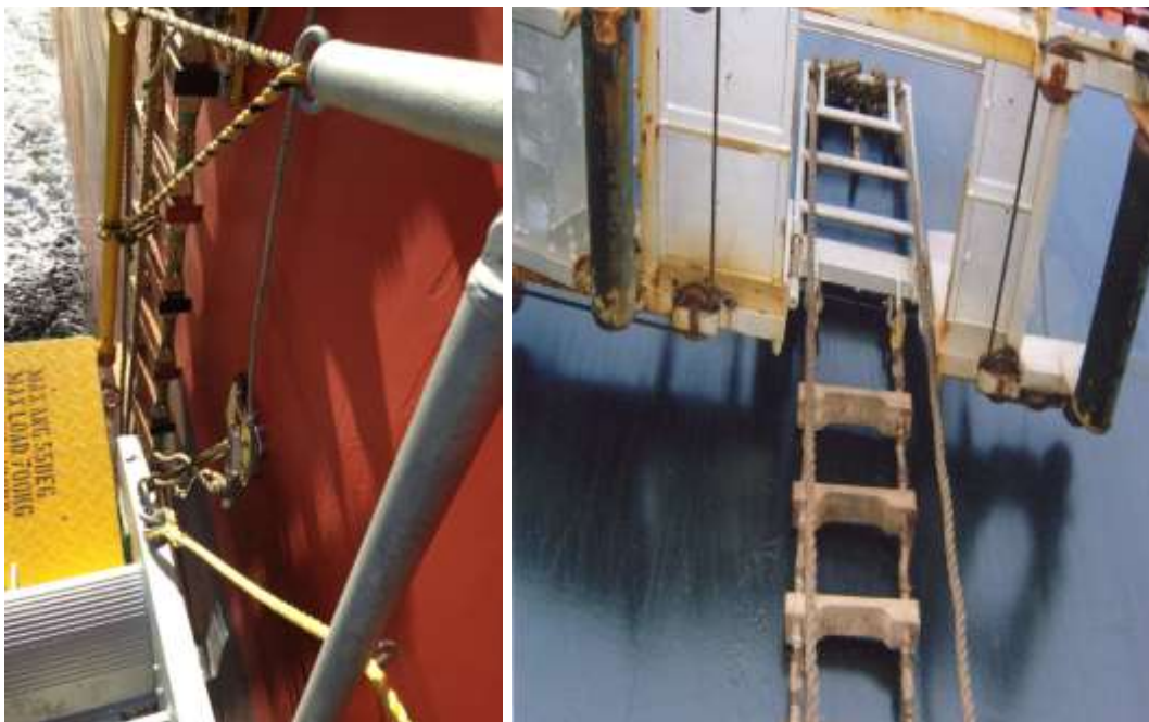
1 Magnet for the Accommodation Ladder NEVER attach ladder to gangway.
